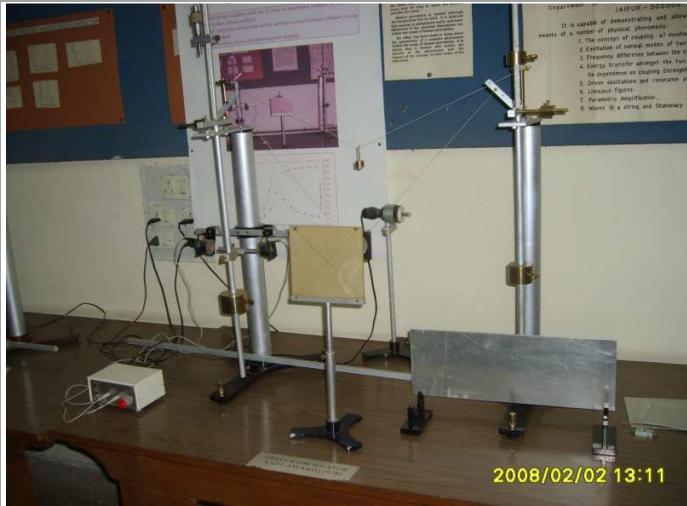
(a) Driven Oscillator System (b) Digital Timer-Two channel (with four sensors)
